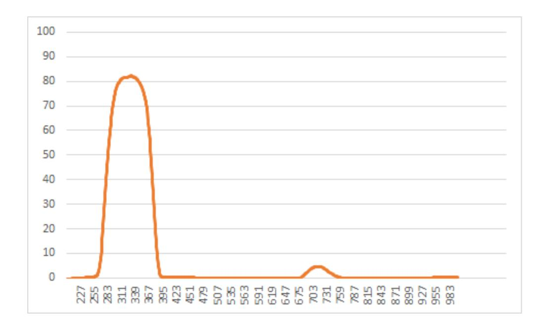
a. UV Reflected image - 0.15% maximum out of band signal
